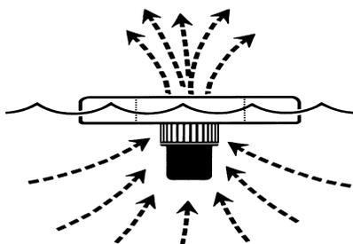
During unit operation, water is circulated from 360° around the unit as well as from below. Top intake for shallow water operation.
