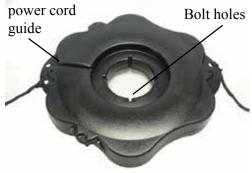
4. Use one of the 1/4"-20 x 3-1/2" Phillips Pan Head Screws (Part 3), one 1/4" split washer (Part 4), and a 1/4" Flat Washer (Part 5) to secure the float. Make sure the split washer goes between the bolt head and the flat washer. Insert screw with washer through bolt hole in float
