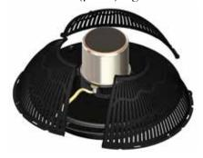
7. Secure the 3 sections of the screen together in 6 places using #8 screw (Part 15), #8 lock washer (part 14), two #8 flat washers (part 13), and #8 nut (part 12). **Do not overtighten.** Alternately, use cable ties instead of hardware for a quicker assembly of the screen.
