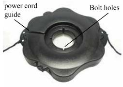
5. Use one of the 1/4"-20 x 3-1/2" Phillips Pan Head Screws (Part 3), one 1/4" split washer (Part 4), and a 1/4" Flat Washer (Part 5) to secure the float. Make sure the split washer goes between the bolt head and the flat washer. Insert screw with washers through bolt hole in float Tighten until snug with a Phillips Head screw driver and repeat for 3 remaining screws.
