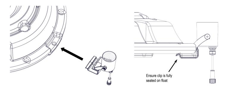
**Step 4**Repeat for remaining fixtures, spacing evenly around the float. Adjust angle of lights using thumb nuts if desired, being sure that the same angle is used for all fixtures. Cable ties can be used to attach fixture cords to float to decrease play and ensure protection. Cable tie light kit power cord to float opposite the fountain power cord for balance and to prevent damage from fountain.
