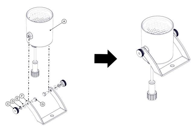
**Step 2**Slide bracket into the top flange on the snap-on clip **(H)** until it clicks into place and is secure.
