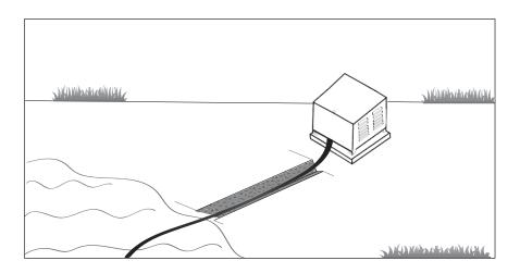
If you live in an area where the water will freeze, you will need to wrap the weighted tubing approximately 4 feet deep into the water with insulation foam. For best results use a closed-cell polyurethane foam.
