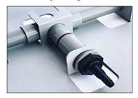
**3.** Slide hose clamp back over tubing and fasten with screwdriver or nut driver.
