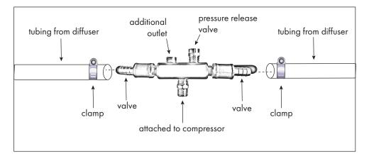
Regulator shut off valves come in a 3/1" barb width. These valves allow you to turn the air on and off, plus they allow you to control the air pressure to each diffuser. When diffusers are different distances away from the air pump, you can adjust the valves so each diffuser has the same amount of bubbling. See image above.
