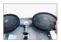
**2.** Slip hose clamp over tubing about 3" and push tubing tightly onto the fitting.
