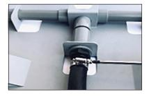
**5.** Screw diffuser(s) onto 3/4" FPT on top of unit. Snug fitting by hand, do not over tighten.
