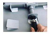
4. To protect the barb and prevent it from breaking while under pressure, fit padded hose clamp over tubing. Use washer. Insert 10mm bolt with washer on both sides of base and tighten nut to clamp down tubing.
