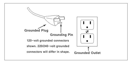
In the event of an electrical short circuit, grounding reduces the risk of electric shock by providing an escape wire for the electric current.
