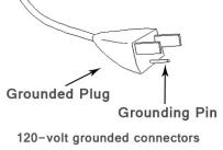
120-volt grounded connectors shown. 220/240-volt grounded connectors will differ in shape.
