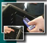
attach the snout. Gently run your fingers along the liner over the area you applied the silicone and flatten the bead out slightly. This will help ensure a more even distribution of the silicone as we compress it while screwing down the snout.
